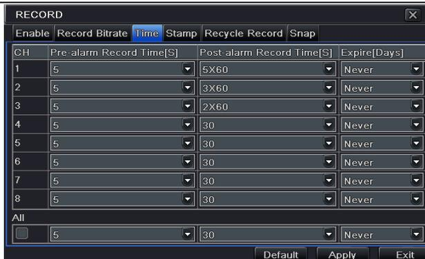
Fig 4-13 record configuration-time
