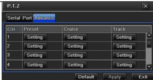
Fig 4-37 P.T.Z configuration-advance
