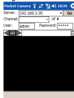
**Step5** : Input the server's address, ID and password respectively in the columns of "Server", "User" and "Password", and click "Go" to log on the server. It will show the picture if access successfully. Refer below picture in the left:
