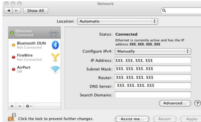
Step 3: After acquiring the IP address, Subnet Mask and so on, please enter into the DVR's Main Menu→Setup→Network interface to manually input IP address, Subnet Mask and Gateway according to the configuration of PC. The network segment should be the same as the PC. If using DHCP, please enable DHCP in the DVR and router.
