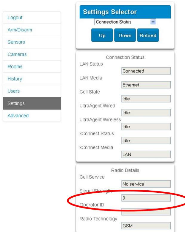
3. Ensure the Signal Strength is -87 to -51 dbm.
