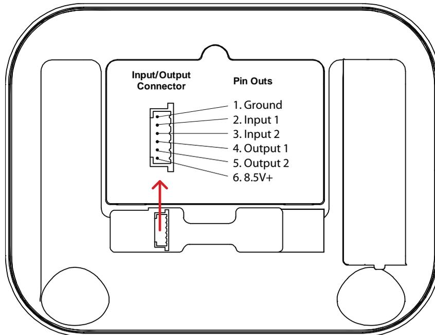
Outputs are controlled by Actions in the ZeroWire.
