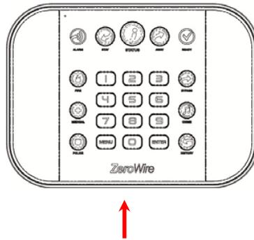
You may enable the box tamper feature from the System Menu – General Options via the ZeroWire Web Server. This will cause an alarm to occur if the ZeroWire is removed from the wall.
