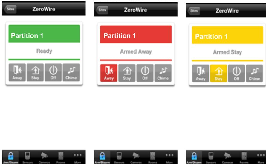
The menu bar is located along the bottom of the app. Touch Sensors to view sensor status. From the Sensors screen you can touch Bypass to ignore a sensor or touch it again to restore it to normal operation. You may also add or remove a sensor from the Chime feature.
