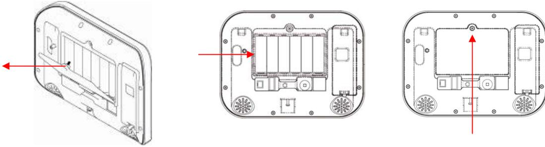
2. Remove battery cover with a small screwdriver.
