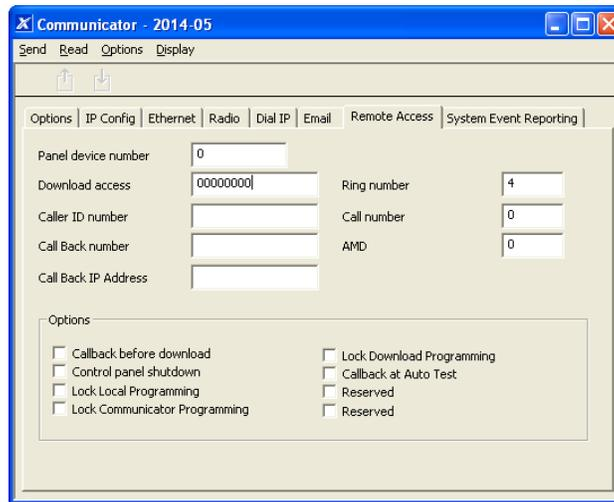
5. Enter the Download Access Code to match the one configured on the ZeroWire panel.
