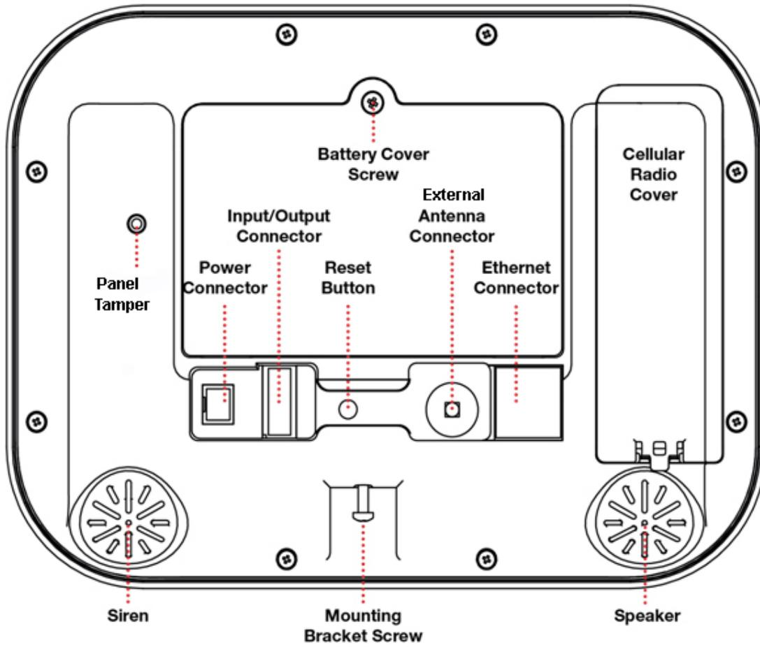
Connections for the cellular radio module are located under the cover on the right.
