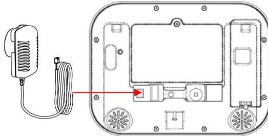
2. Connect the power pack to its own power outlet and turn it on.
