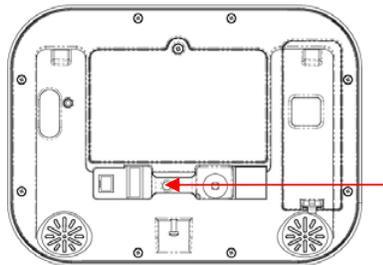
2. Wait 3 seconds after turning on the power, then release the reset button. This will reset user 40 to PIN 9713 and username "installer".
